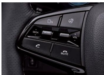
Remote controls switches and cruise control system on the steering wheel
