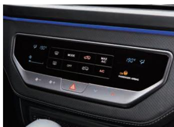
Dual-zone fully automatic/manually controlled air-conditioning
