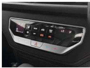
Manual Control air-conditioning
